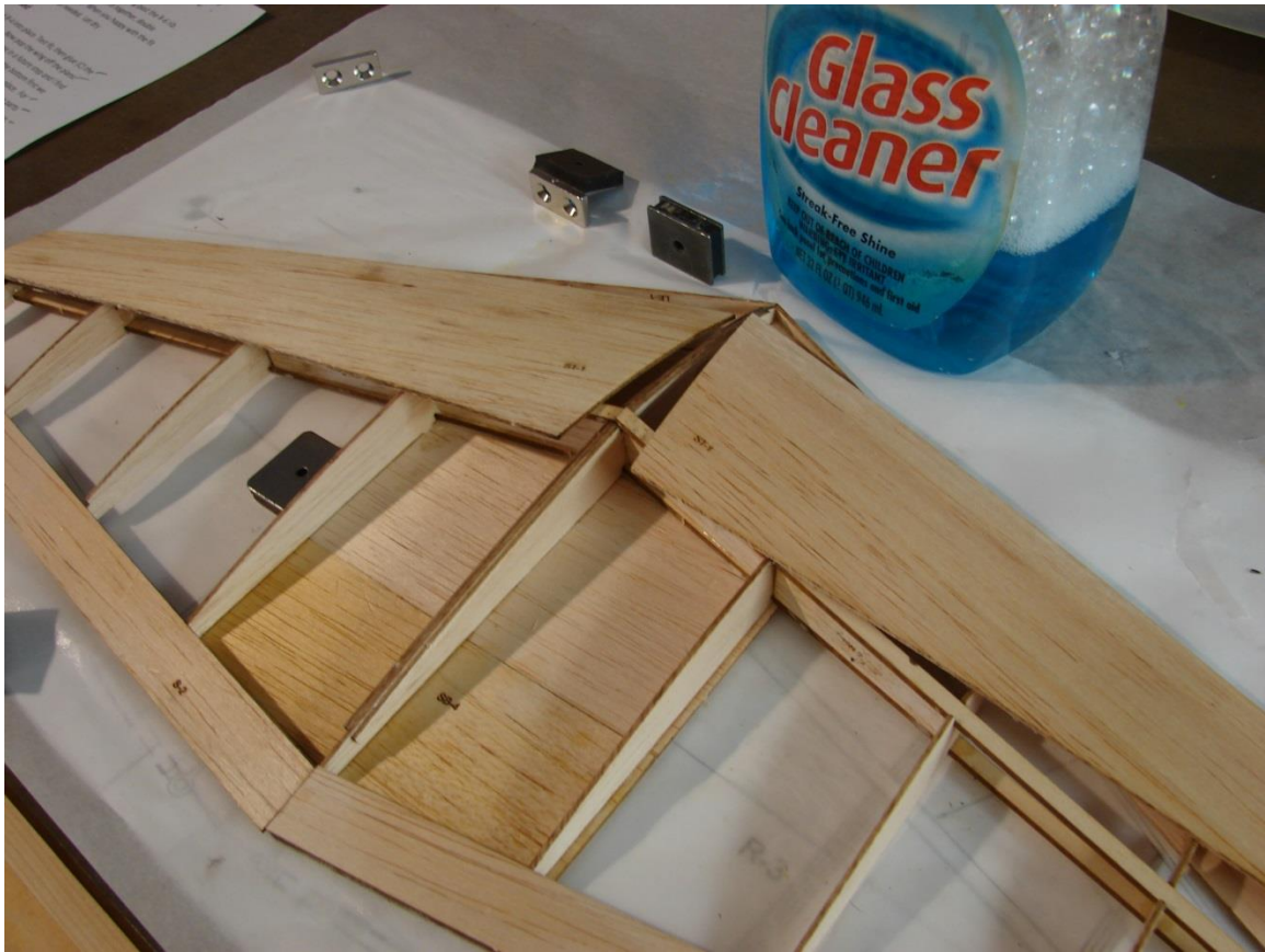
Glue (C) the ST-4's into place. Dampen the ST-1's and Glue (C) to the top leading edge.
