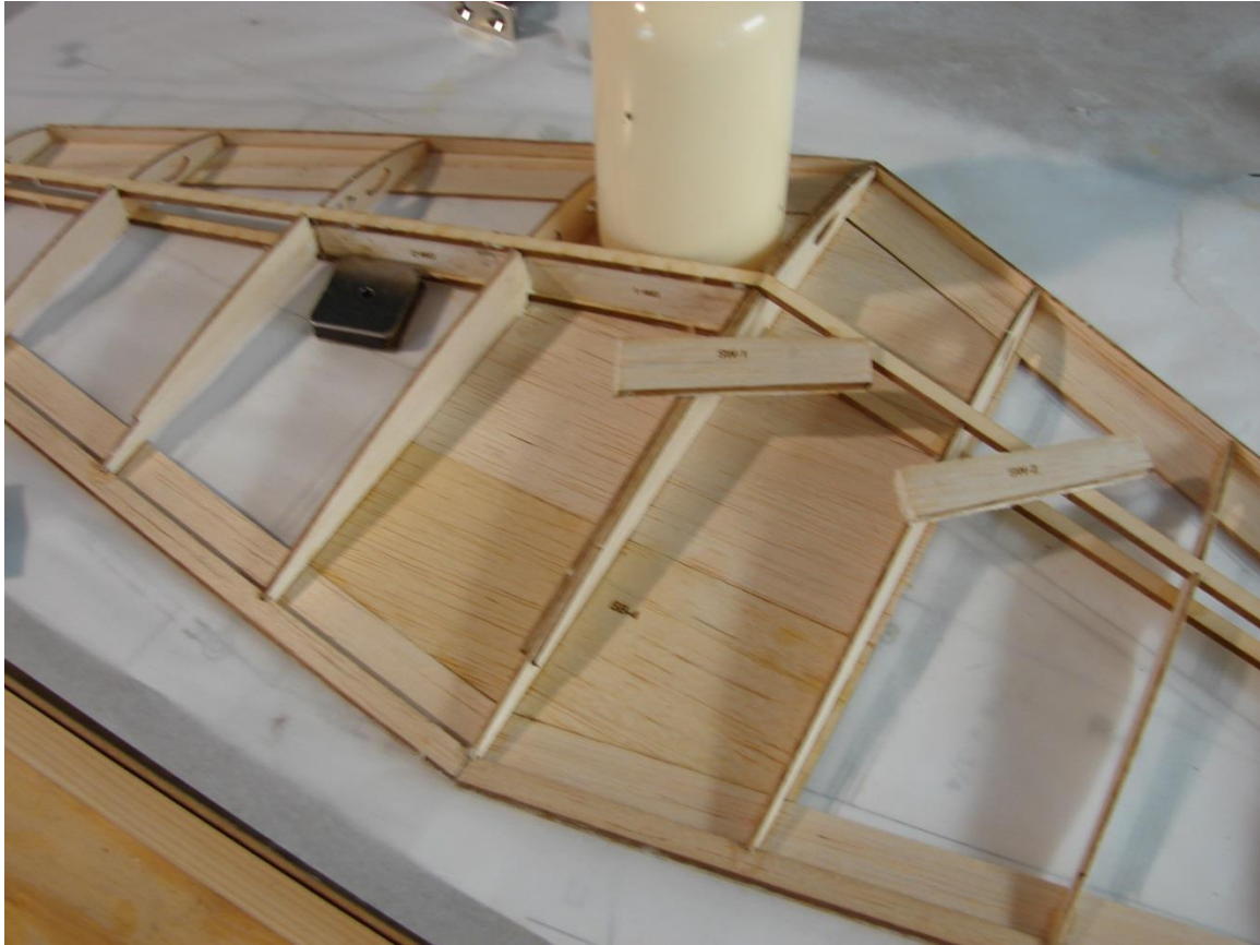
Test fit & glue (A) SW-1, SW-2 shear webs in place.
