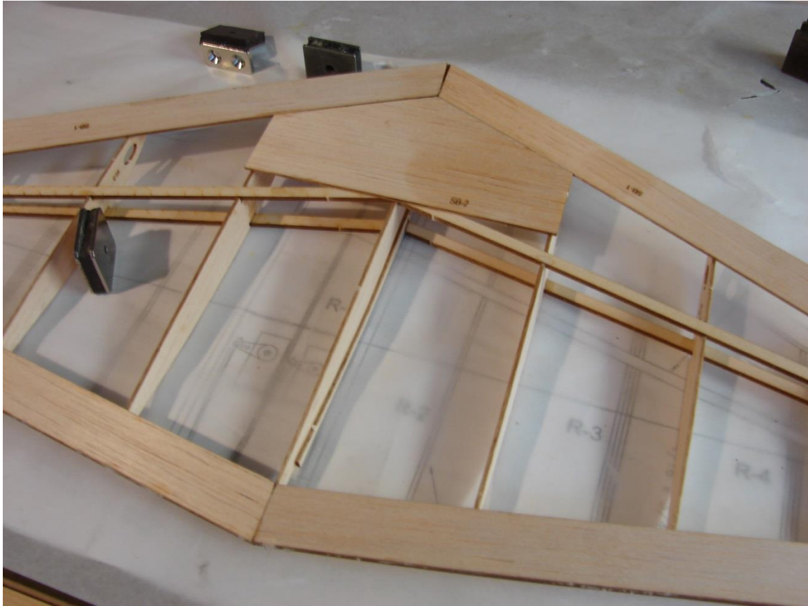
Bottom of the Wing: SB-1, SB-2 & ST-4 trailing edge sheeting in place.
