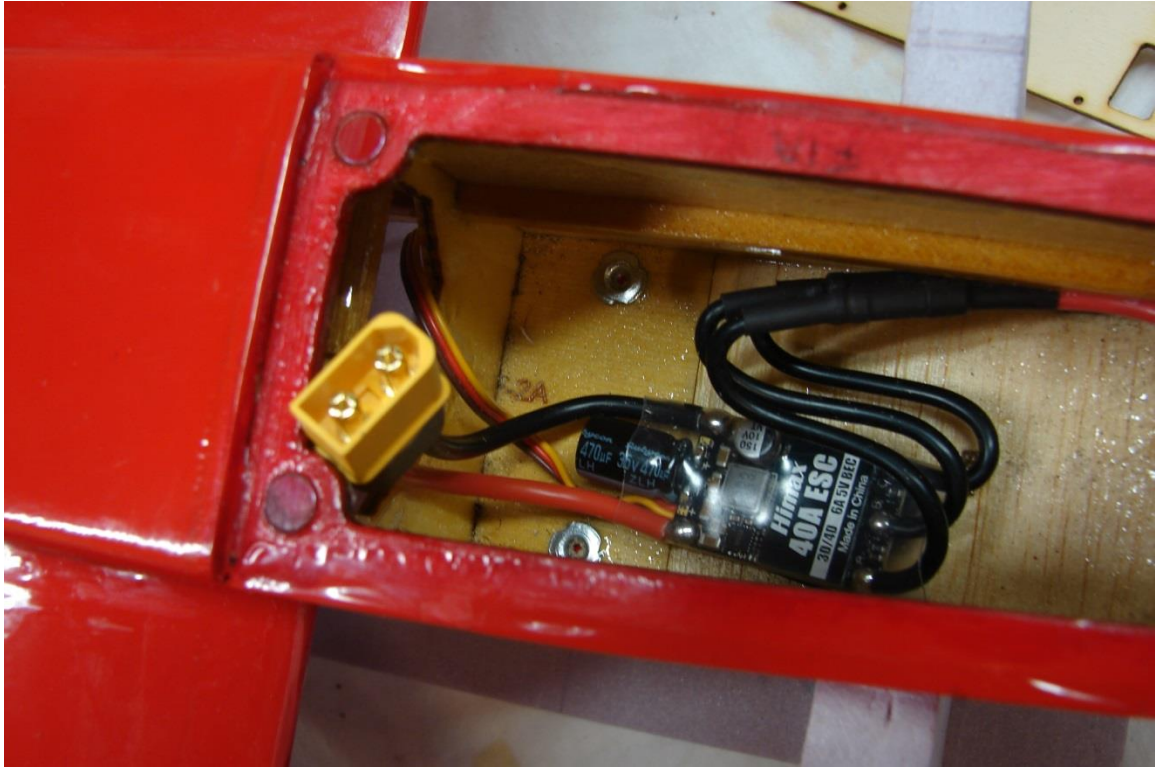
Esc Velcro to the floor, connector faces rearward, "S" bend on the ESC wires.
