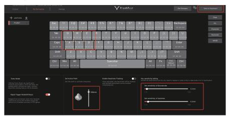
After you select the key you want to adjust the sensitivity of, drag the white dot to select the point you want the key to be triggered, then click the "Save to keyboard" button to save it.
