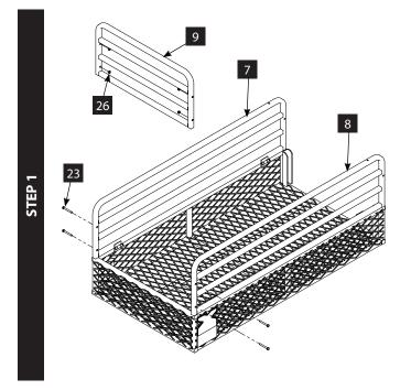
1. Fold side rail left and right (7 & 8) up and attach front rail (9) to both side rails using four 5/16-18 x 2-1/2 IN bolts and nuts (23 & 26).
