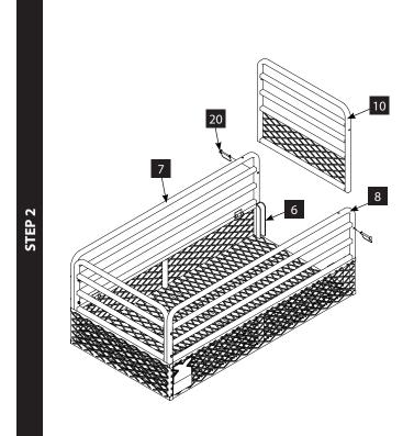
2. Slide removable tailgate (10) into the brackets of the trailer bed (6) and secure to left and right side rails (7 & 8) using two  $\frac{1}{4}$  x 3 IN snap pins (20).
