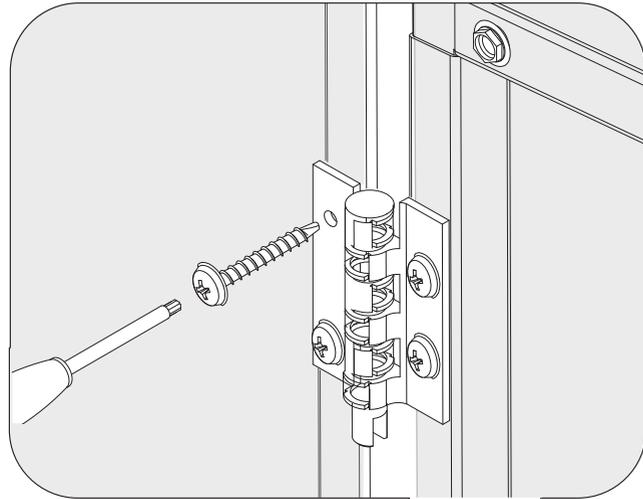
EN Mount the hinge on the polycarbonate board.
