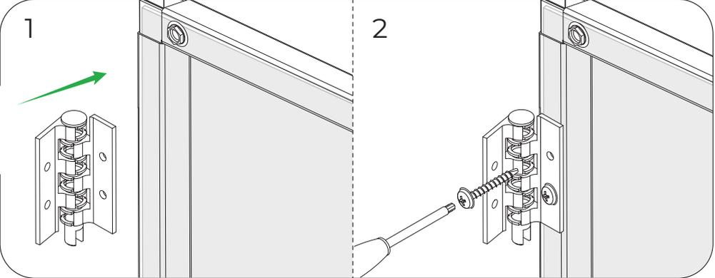
EN Mount the hinge on the polycarbonate board. Left and right hand side assembly is possible.
