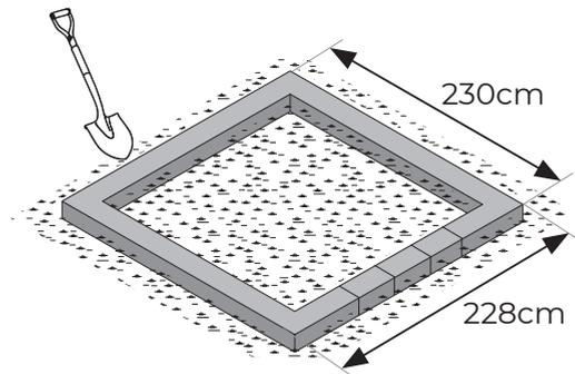
standard concrete block 24x12x38 weight approx. 22-25kg
