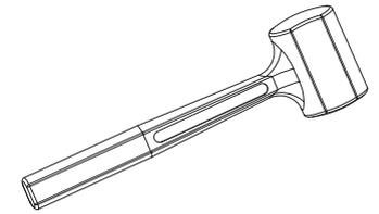
EN Hammer in the profiles with a rubber hammer (not a steel one)
