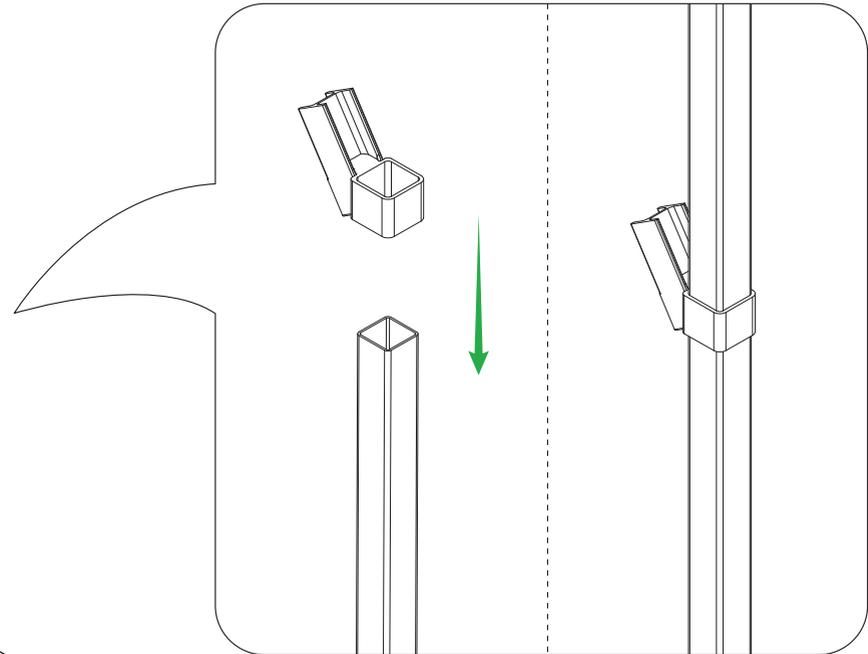
EN About 710 mm from the ground to the connector Z-11A
