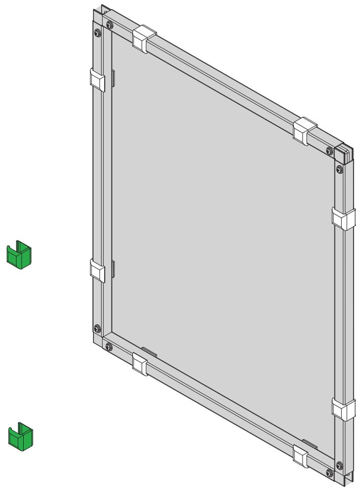
! EN All Z-14 clips must be fastened with W1 screws from the inside of the greenhouse.
