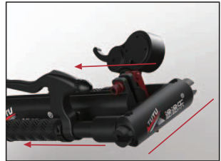
Step 3: bend the handle downward
