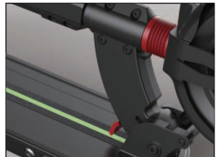
Step 6: push forward and at the same time hold down the lever when folding the head.
