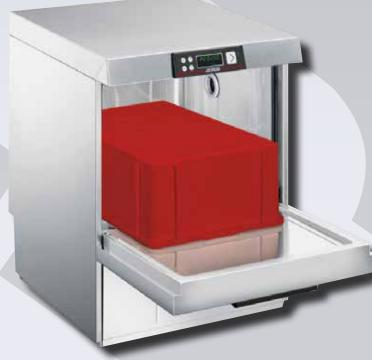
Double skin construction in AISI 304 stainless steel with insulation. Moulded tank with rouned corners. Balanced and insulated door with gasket. 2 rotating wash arms with 8 nozzles each and 2 rinse arms with 7 nozzles each, which is made of stainless steel, ensures optimum washing results.
