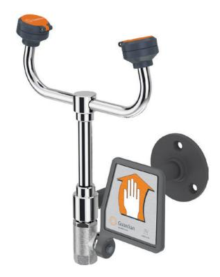
**Application:** Eyewash for wall mounting. Two GS-Plus™ spray-type outlet heads deliver a flood of water for rinsing eyes. Unit is provided without bowl or drain for waste water. Note: Floor drain should be provided underneath unit to prevent accumulation of water on floor.
