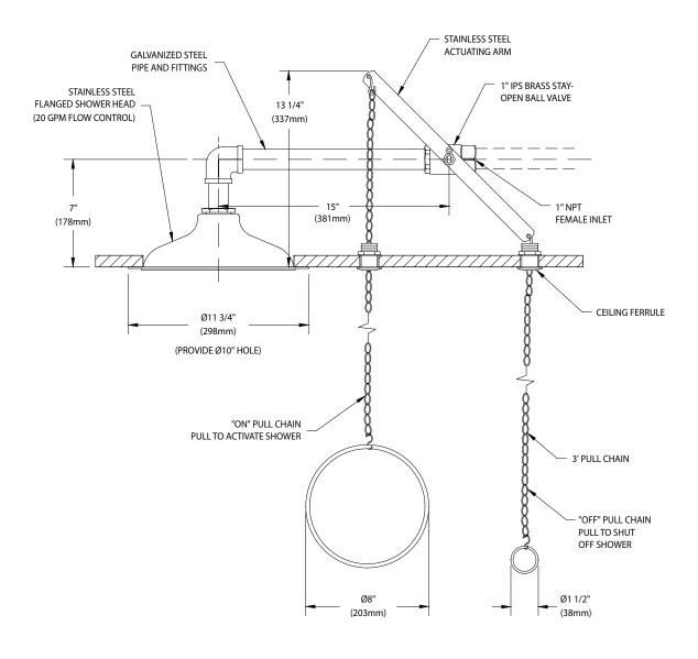
UNIT IS DESIGNED FOR MOUNTING IN 8 FT. CEILING
