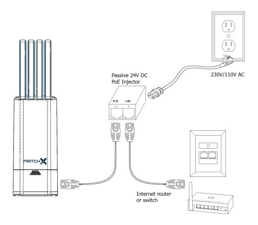
Figure 2.1: Connection of MX1901/2 Gateway.
