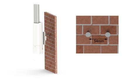
Figure 2.2: Mounting the MX1901/2 Gateway to the wall.
