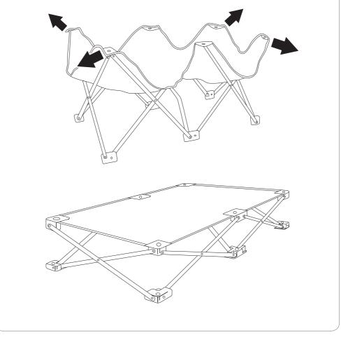
**NOTE:** Check that the bed is opened as far as possible and that there are no loose parts before use. The bed will not fully lock into place until use, when there is weight on the surface.
