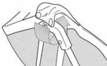
Wrap hinge cover flap over then under the hinge and snap to inner side of the hinge. Repeat for remaining hinges.
