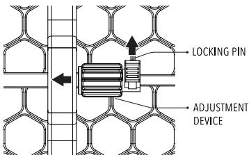
To lock the gate into position, pull up on the locking pin and slide the adjustment device towards the center of the gate.
