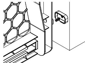
Reinstall your gate in the doorway or opening according to the instructions, using the newly installed wall cups as anchoring points for the (4) rubber bumper.
