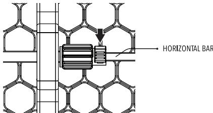
When the adjustment device can go no further, push down on the locking pin. The pin will insert into one of the holes on the horizontal bar and secure the adjustment device in place.
