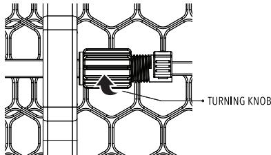
Use the turning knob to tighten and secure the gate in place. Rotate the knob away from you (clockwise) until enough pressure is created to stabilize and secure your gate.
