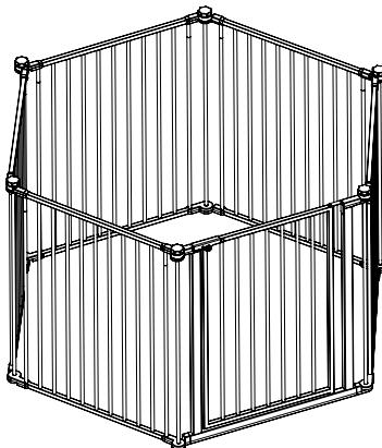
**NOTE:** When adding or removing additional panel units to the configuration, panels must be added or subtracted in sets of two for the freestanding enclosure to function properly. ADDITIONAL PANELS SOLD SEPARATELY.
