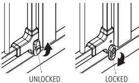
To open the gate, start with rotating the base lock in the upward direction. Do this on both sides of the door.
