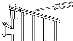
Use a Phillips/crosshead screwdriver to fix the wall mounting bracket to the wall. Repeat for all four brackets.
