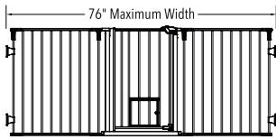
Arrange the panels to your desired configuration, then tighten all of the hinge knobs.
