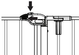
Press the release button down on the handle. Slide the handle back towards the hinge.
