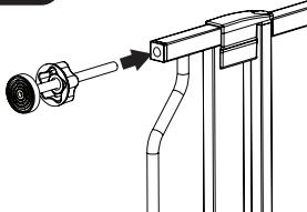
Insert the (4) threaded spindle rods into the holes at each of the four corners of the gate.
