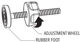
Locate the (4) threaded spindle rods (F). Rotate the adjustment wheels along the threading, eliminating the gap between the adjustment wheel and the rubber foot.
