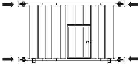
Insert the (4) threaded spindle rods into the holes at each of the four corners of the gate.
