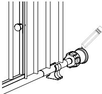
After you have mounted your gate, and you are satisfied with its positioning, draw a circle on the surface of your doorway or opening around the perimeter of the (4) rubber feet.
