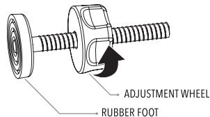
Locate the (4) threaded spindle rods (E) Rotate the adjustment wheels along the threading, eliminating the gap between the adjustment wheel and the rubber foot.
