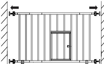
Position the gate so that it is level and centered within your doorway or opening. Rotate the adjustment wheels on the threaded spindle rods in the opposite direction as in Step 2, expanding the gap between the rubber foot and the adjustment wheel. Expand each of the (4) threaded spindle rods until they make contact with the doorway or opening. Do not fully tighten the threaded spindle rods yet.
