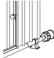
Reinstall your gate in the doorway or opening according to the instructions, using the newly installed wall cups as anchoring points for the (4) threaded spindle rods.
