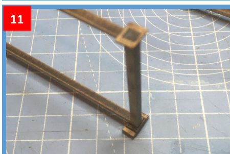
11 Glue the pads (9) to the bottom (the thicker frame), of the support frame
