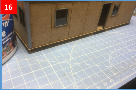
16 Fit the glazing using a small amount of glue to ensure there is no "squeeze out"
