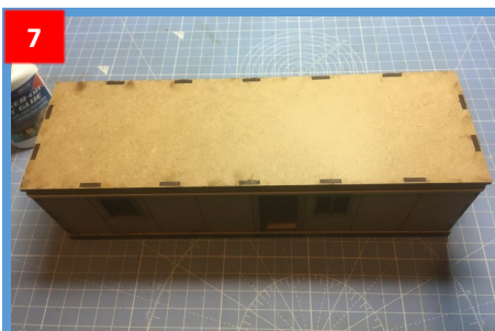
7 Glue the roof (6) to the walls
