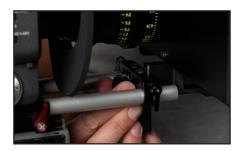
1 Loosen the knob on the rail block
