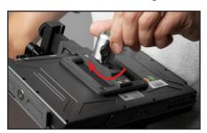
① Attach the 16mm adaptor to the 3/8" threaded hole in the base of the ZeePrompt.
