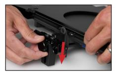
• Move the railblock to its lowest position and secure using the knob.
