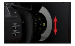
2 Position the ZeePrompt so that the lens is positioned in the centre/uppercentre part of the hole.
