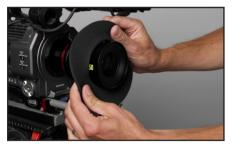
2 Choose a suitable doughnut and fit around the rim of the lens
