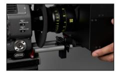
3 Loosen the two levers on the rail block. Slide the ZeePrompt onto the bars. The front of the lens should be in line with the hole in the main box, (or pushed through to the beamsplitter glass if a wider focal length is needed). Re-tighten the two levers and rebalance your tripod head accordingly.
