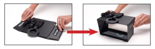
Use both hands to unfold the main unit. NOTE: It may not fully lock into place until attached to your computer.
