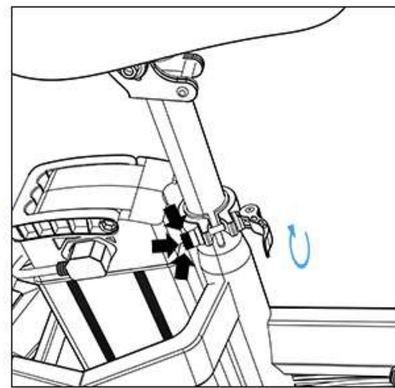
3. Clockwise rotate the quick-release lever with one hand holding the adjusting nut.
