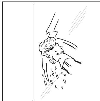
Step G Applying Silicone Sealant And Cleaning Seal from the top of the wall channel to the bottom on the Outside between the wall channel and the wall, and between the bottom profile and shower tray as shown. Wash down with clean warm water and a soft clean cloth or sponge. Please do not use bleach, alkaline or acid-based, aggressive or abrasive cleaning products.
