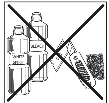
Step G Applying Silicone Sealant And Cleaning Seal from the top of the wall channel to the bottom on the Outside between the wall channel and the wall, and between the bottom profile and shower tray as shown. Wash down with clean warm water and a soft clean cloth or sponge. Please do not use bleach, alkaline or acid-based, aggressive or abrasive cleaning products.
