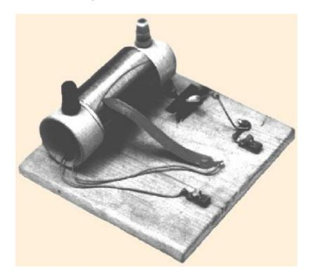
The design below came from a submission by Lt. Paul M. Cornell in the September, 1945 issue of QST; he used it in the South Pacific. The photograph shows a similar radio built by Don Menning; he simply stuck the whole tip of a pencil on the end of the safety pin.
