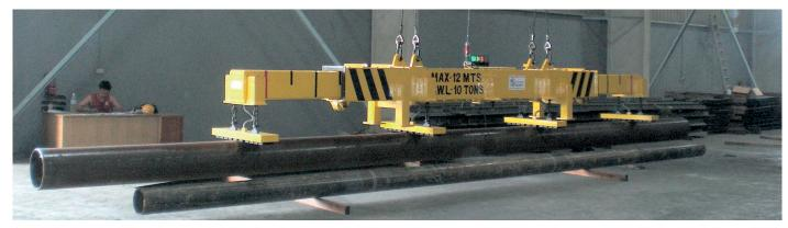
ElectroPermanent Plate Lifting Magnet
