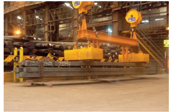
25 Ton Billet Lifter undergo load test
