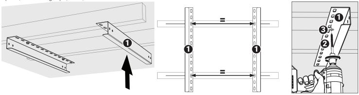
**b)** Screw in the remaining slots, and test the fit using an empty storage bin.
