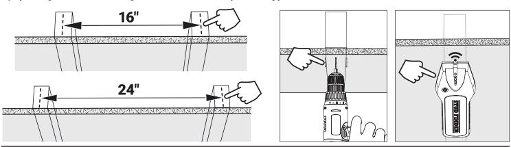
b) When found, mark the edges and center of the ceiling joists.
