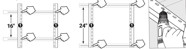
a) Screw the rail using the lag bolts and washers provided in the installation kit (DO NOT OVERTIGHTEN).
