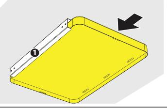
**b)** Slide the second rail on top of the lid and mark the appropriate mounting slots.
