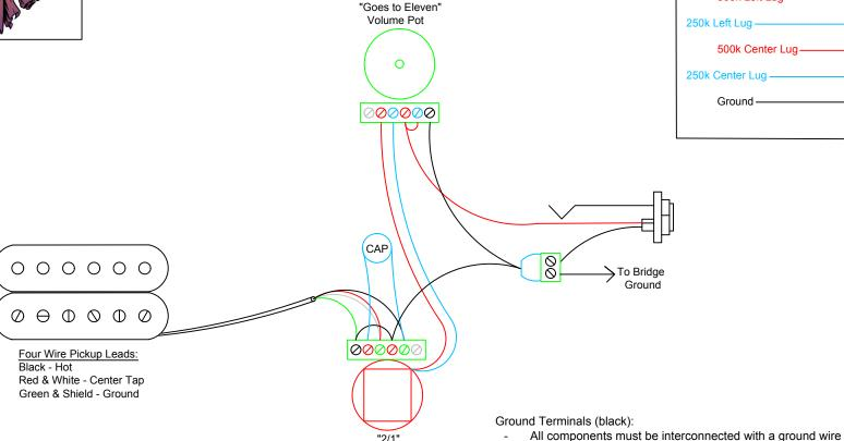
Pickup wire colors may differ than yours. See "Pickup Cross Reference Chart" at madhatterguitarproducts.com to verify your pickup wire color configuration.
