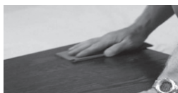
SANDING #120-#150 GRIT WITH THE GRAIN
