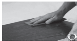
SANDING #120-#150 GRIT WITH THE GRAIN
