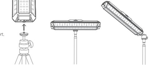
Caution When you connect MULTI FACE X and lantern stand, do not fix screws on both sides of the body, stand can be fall down.
