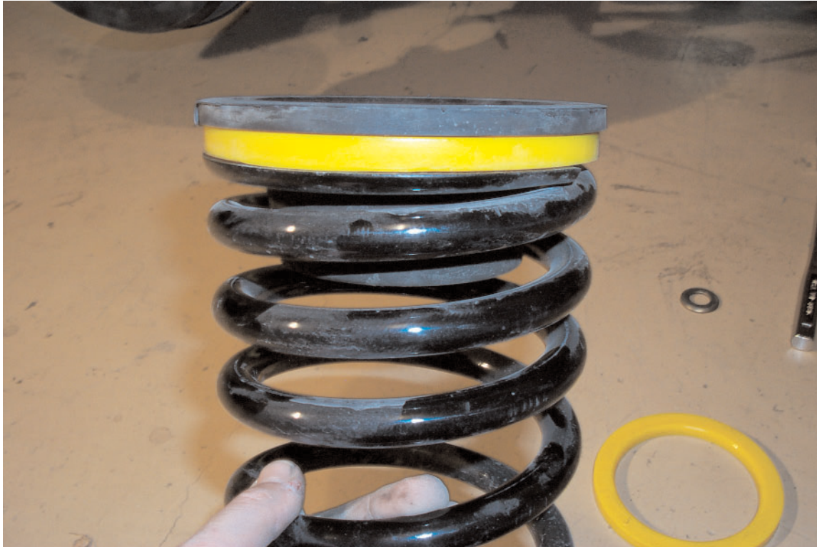
Old Man Emu 890 Coil with 10mm Trim Packer and Cone installed.
