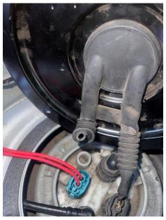
5. After the wires are fed through the grommet and you've connected the fuel pump connector you are going to plug the wires into pins 2 & 4 on the BLACK EKPM connector. (make sure you hear a click to confirm it is fully inserted). Once the connection has been made make sure to put the locking tab back into place.
