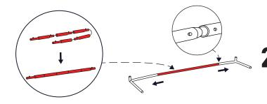
Unfold the horizontal pole. Attached the horizontal pole to the two L-Shaped
