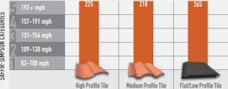
ASCE 7-10 Wind Design Standard. Exposure C, 30 foot mean roof height, Large paddy, Importance factor 1.00, High Profile based on a tile factor of 1,407, 2:12 to 6:12 slope, gable/hip roofs.
