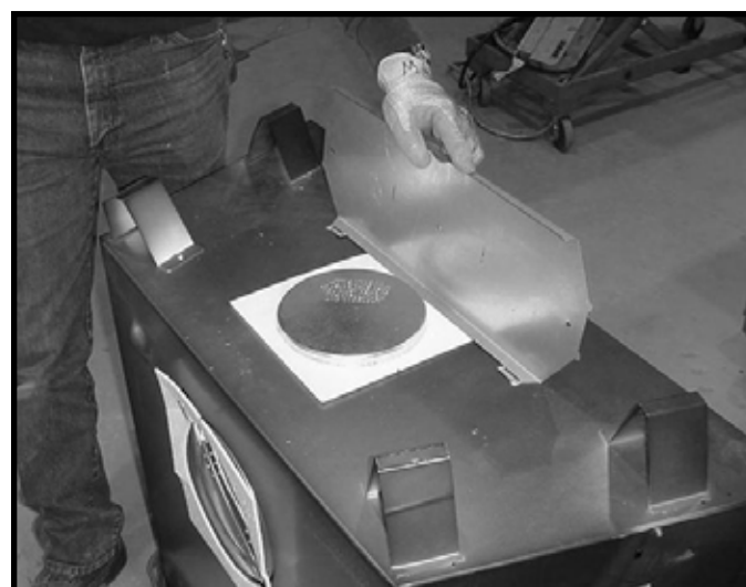
Figure 6.6 Rotate the top heat shield to the vertical position as shown above. The heat shield must remain in the vertical position.
