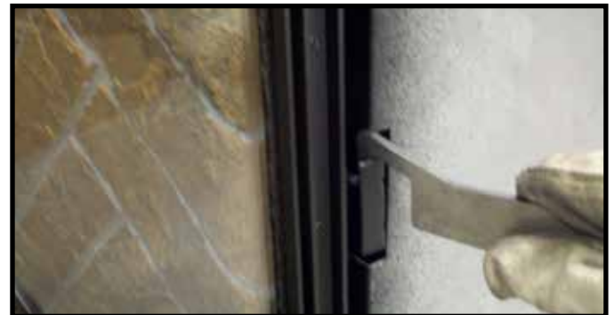
Figure 11.7. Securing Side Glass Clips
