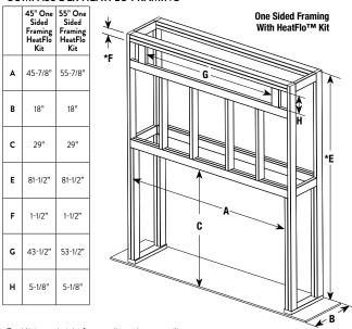
${\sf E}$  = Minimum height from appliance base to ceiling  ${\sf F}$  = Minimum opening distance from ceiling to allow for min distance from HeatFlo register to ceiling of 6"
