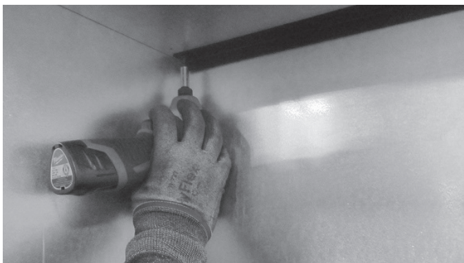
Figure 7.2 - Remove Rear Black Magic Glass Bracket
