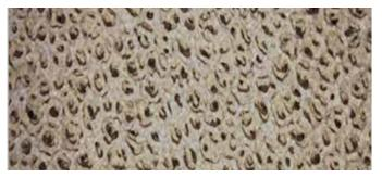
Combustor Problem - Ash, a fluffy light grey powder, and soot, accumulate on the combustor surfaces in normal use. In extreme situations combustor can become clogged and should be cleaned.
