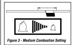
For instance, a long chimney will necessitate closing the damper more. To obtain the proper combustion, close the damper completely, then open it about 1/2" to 3/4". Three medium size pieces of cord wood-burning on a bed of hot coals will generate an approximate heat output will of 35,000 BTU per hour and the loading time will be about every 3-4 hours.
