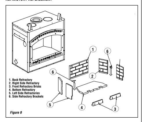
The intense heat of the fire will normally cause hairline cracks in the refractory brick. These cracks can be minimized by proper curing as described in section *First Fires*. They will not normally diminish the effectiveness of the refractory brick. If large cracks develop, then the refractory should be replaced. To replace the refractory bricks, follow these steps:
