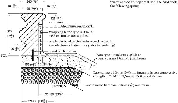
Allow 6mm  $(\frac{1}{4})$  for vertical and bedding joints Unless otherwise stated, all materials other than stonework to be supplied by others
