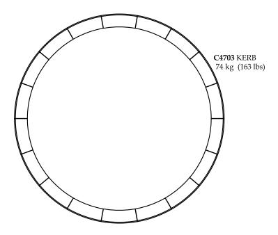
$\emptyset$  10mm ( $\frac{3}{8}$ ") stainless steel dowels (not supplied) 50mm (2") projection into stone. Holes to be drilled on site to suit by others. Minimum of 2 No dowels per stone secured using a flexible building adhesive such as Evode Serious Stuff, Loctite Fast Grab, or similar
