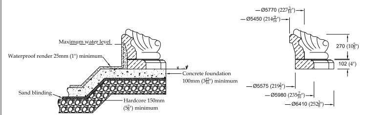
Read in conjunction with tech Sheet P11, P12 and P50 All dimensions exclude joints - allow 6mm  $\binom{1}{4}$ ") for vertical and bedding joints Unless otherwise stated, all materials other than stonework to be supplied by others
