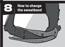
Remove the sweatband by detaching it from the hooks. To replace, simply align the new band and hook in place.
