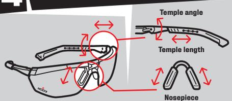
The multiple adjustment settings help the glasses fit your face securely and comfortably. Adjusting the temple angle can also control the airflow.
