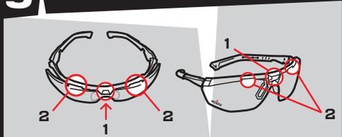
Always ensure that the lenses are properly attached to the frames before using the glasses. To do so, begin by attaching the middle point of the nose and then attach the right and left clips.
