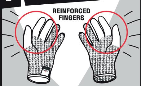
Made of ultra high molecular weight polyethylene, glass fibre, nylon, polyester and spandex. The 3 fingers are reinforced with stainless steel threads.
