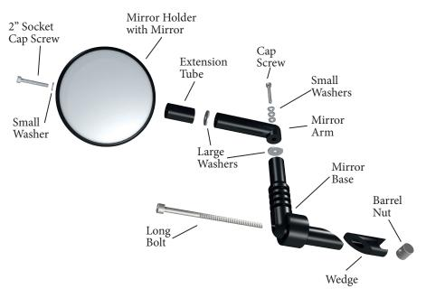
The extension tube kit may be used between the mirror base and mirror arm or between mirror arm and mirror holder.
