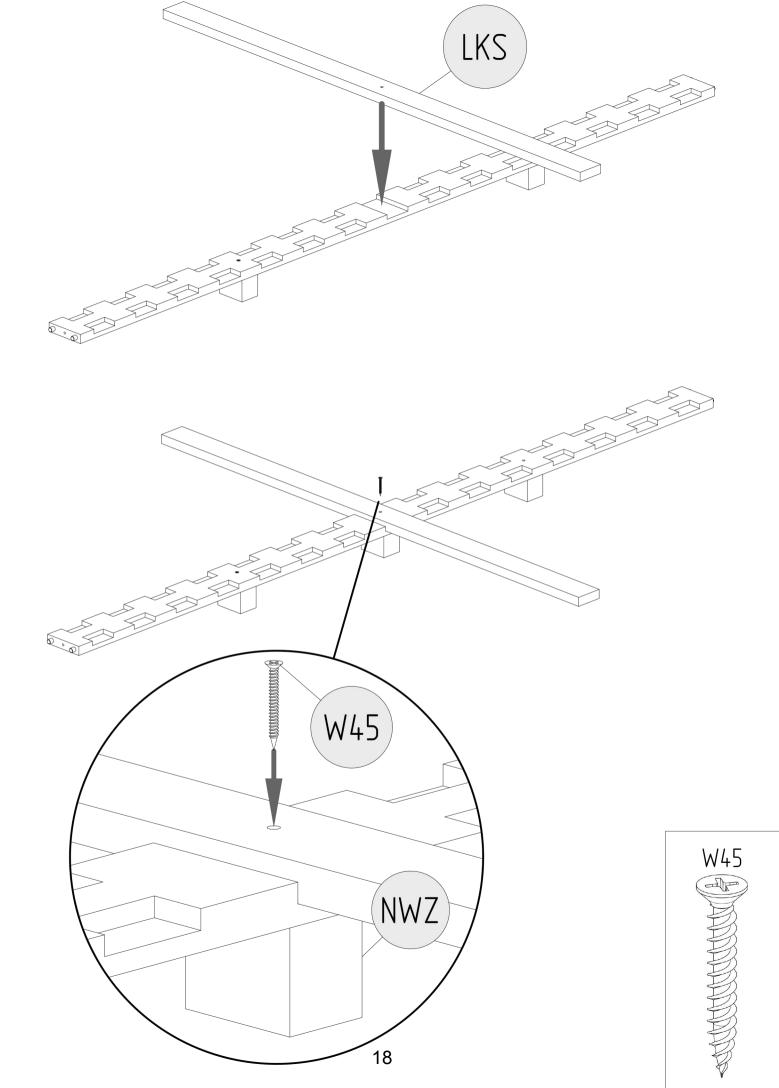
TO PROPERLY SCREW DOWN THE BED LEG, SEE THE FIRST PART OF THE MANUAL
