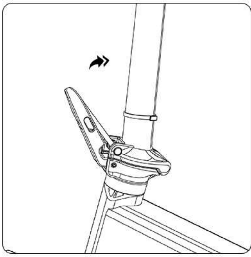
19. Fold the foldign handle of the headset stem.
