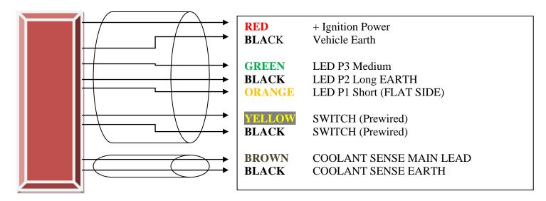
Red: 8 to 30Vdc (switched power), Use the cable joiner to Tee into a positive ignition wire.
