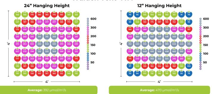
PPFD readings were taken in an Active Grow Walden Tent 4'x4' using Active Grow 25W T5 HO Ballast Bypass 4FT LED Grow Lamps in Sun White Spectrum and an Apogee Extended Range PFD Sensor.
